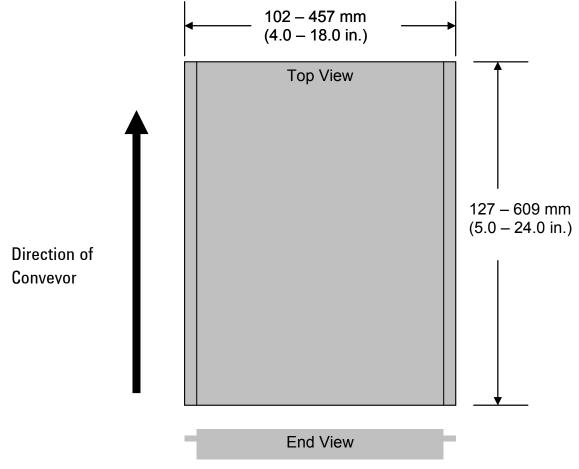
Maximum carrier height above top conveyor surface: 9.4 mm (0.37 in) Maximum carrier height below top conveyor surface: 30.0 mm (1.2 in.) Maximum weight of loaded carrier:4.5kg (10 lb.)
