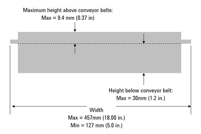
The carrier flanges protrude from the sides of the carrier and allow it to be carried by the conveyor and secured by the clamps in the 5DX.
