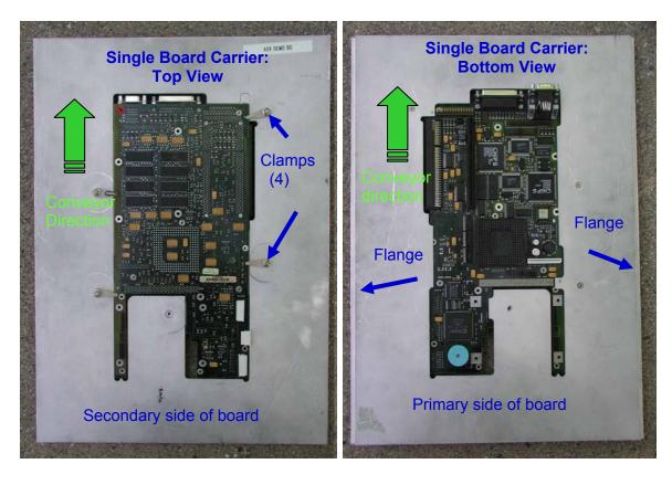
**Case 1:** The board shown above is tested with the primary side of the board toward the bottom of the 5DX. Several of the connectors and other components are taller than allowable for top side clearance.
