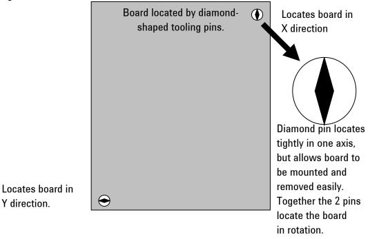
Placement of the tooling pins for each board relative to other boards is also critical in order to position the boards on the carrier where the 5DX program expects them.
