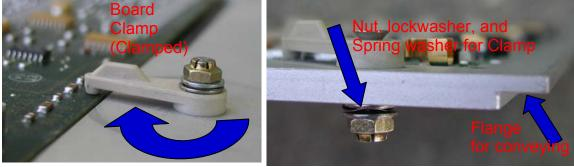
**Case 1**: Boards are sufficiently flat for x-ray testing (< 1% warp in any linear dimension) Small hold-down clamps are usually sufficient to prevent board motion during test.
