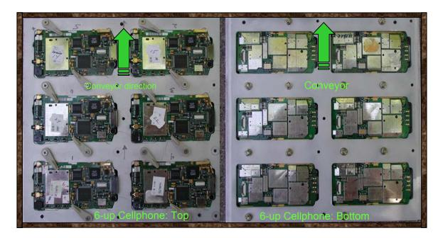
**Case 3**: An example where high production throughput is required from the 5DX, and the boards are small enough that several can be put on a carrier.
