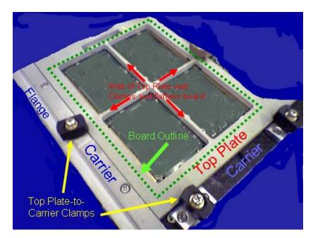
**Case 2:** A top plate or other system of clamping the boards to the carrier will prevent the boards from moving during test, and can reduce false calls and the need for additional surface map points by flattening the boards. A portion of such a carrier is shown in detail.
